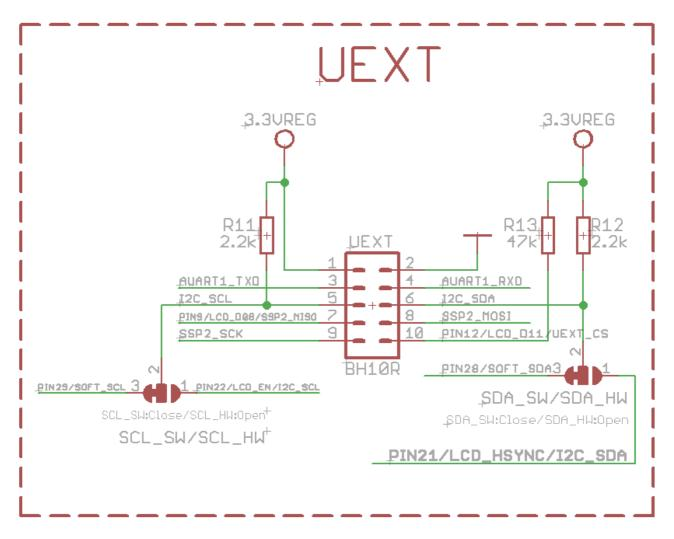
\*Note the two jumpers PIN29/SOFT\_CL – PIN22/LCD\_EN/I2C\_SCL, and PIN28/SOFT\_SDA3 – PIN21/LCD\_HSYNC/I2C\_SDA which by default are set to a software SPI. They can be used to set the whole UEXT to a hardware SPI.
