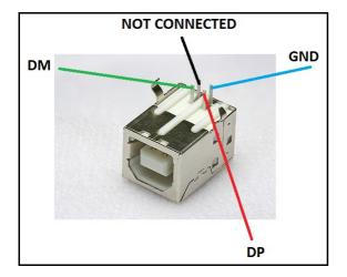
After soldering the three wires you can place a marker on each of them or use colored wires to be able to distinguish them. You can also use some gel to keep them tight on the USB connector. On the opposite side of the cables you might place 50mil (1.27mm) male connector following the order of the signals. Please also restrain from using wires longer than 20 cm since that might make the connection unreliable.
